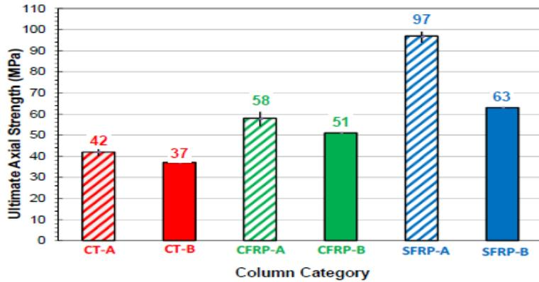
Figure 1. Ultimate axial strength of Group A and Group B specimens
