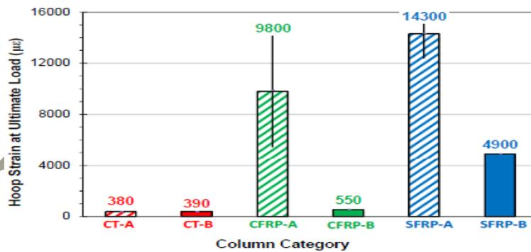
Figure 3. Hoop strain of Group A and Group B specimens
