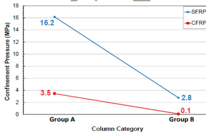
Figure 5. Confinement Pressure of Group I and Group II columns
