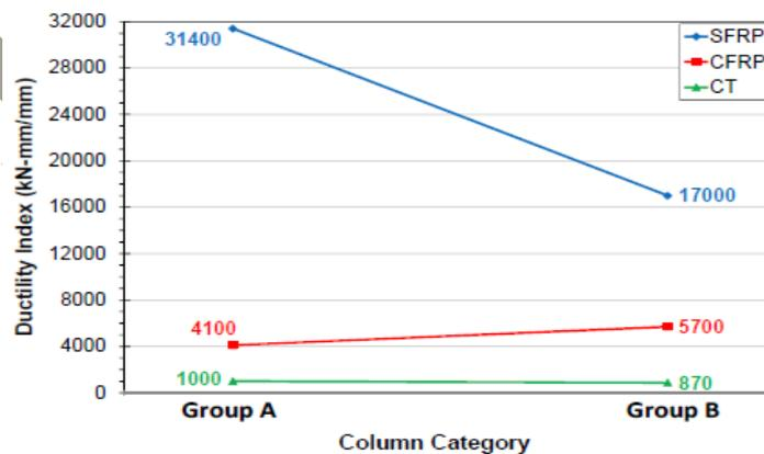
Figure 4. Ductility of Group A and Group B specimens
