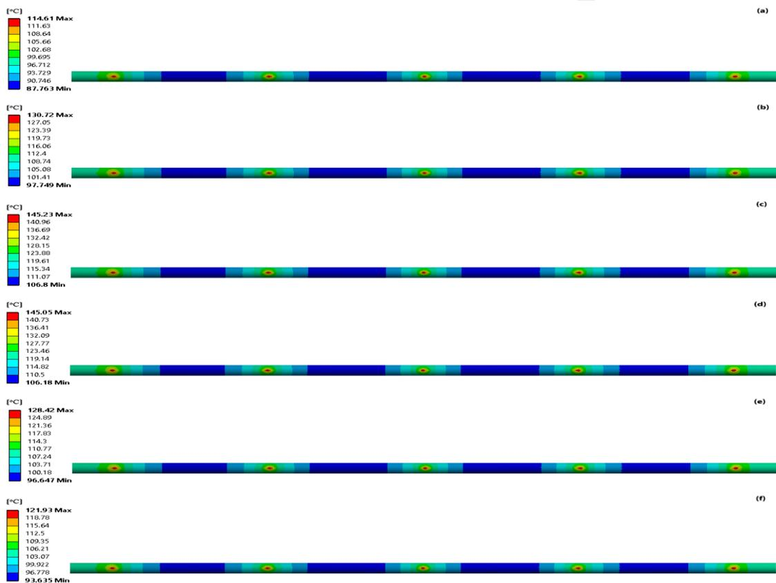
Figure 6 Temperature distribution on heat exchanger surface at (a) Re 10000, (b) Re 9000, (c) Re 8000, (d) Re 7000, (e) Re 6000 and (f) Re 5000
