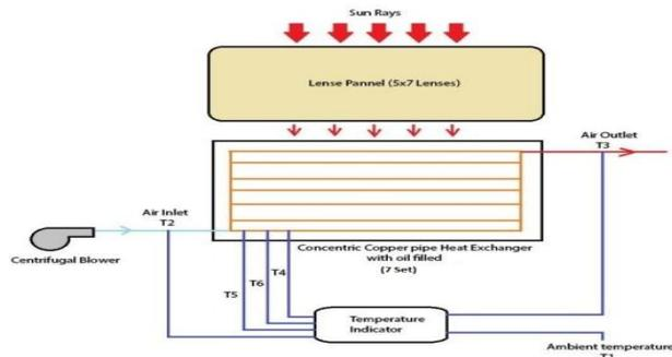
**Figure 1 Schematic view of setup**
