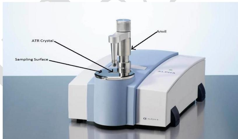
**Figure 2. Bruker Alpha - E Spectrometer**
