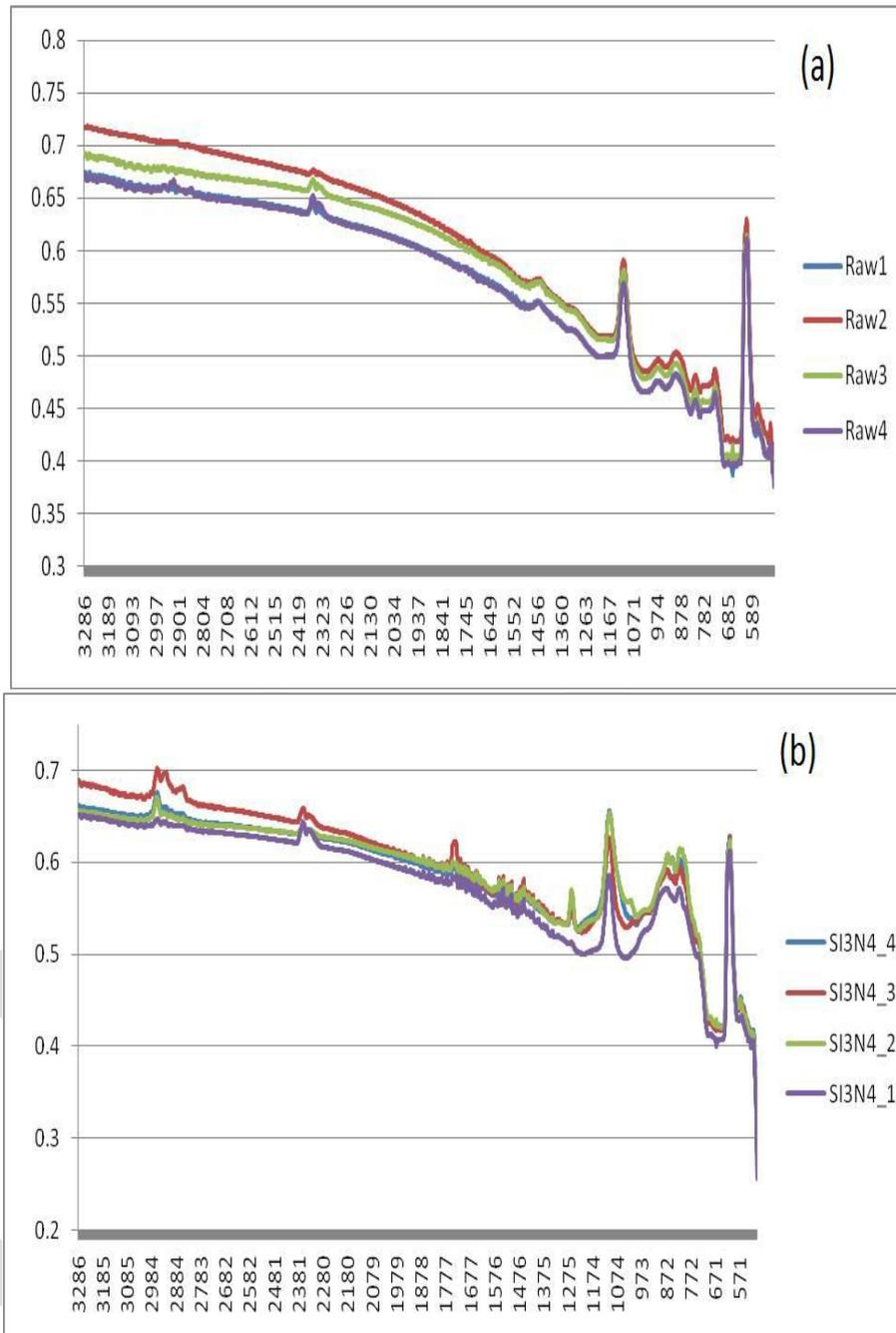
**Figure 3. FTIR GRAPH of IC Grade Mono crystalline Wafers: (a) Raw Wafers & (b) Silicon Nitride coated Wafers**
