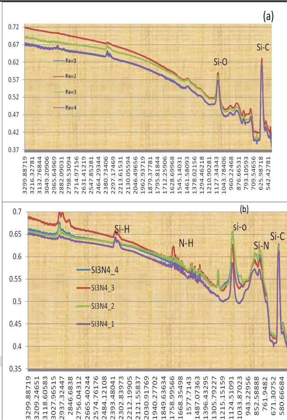
**Figure 4. FTIR GRAPH of SIN Solar Grade Wafers: (a) Raw Wafers & (b) Silicon Nitride coated Wafers As can be inferred from the above graphs, the coating of silicon nitride increase the absorptivity around 853 nm from 0.45 to 0.58. It can be inferred that the above process can bring about 28% increase in absorptivity.**
