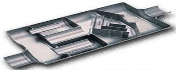
**Fig. 1.1 A Reactive Muffler**
