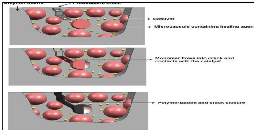
**Fig 3.1: embedded microcapsules.**
