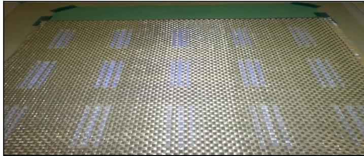
**Fig 4.1: Solvent-epoxy filled (with a fluorescent dye) HGFs glued on E-glass fiber sheets before infusion of the resin and hardener mixture.**
