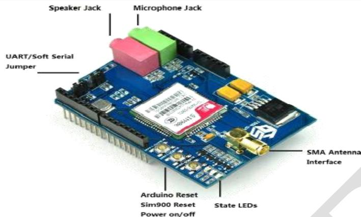
Fig .6 GSM Board
