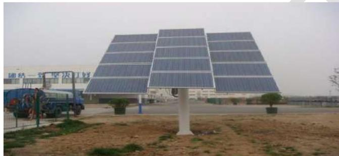
**Fig: 1.5.2.c) Vertical Axle Tracker**
