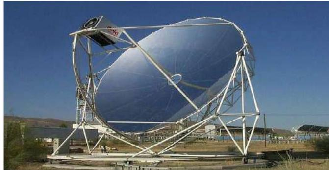
**Fig: 1.5.2.e) Two Axis Mechanical Mount type Tracker**
