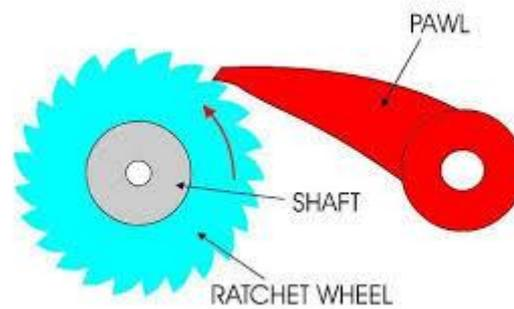
**Fig.3 Schematic of Ratchet Pawl**
