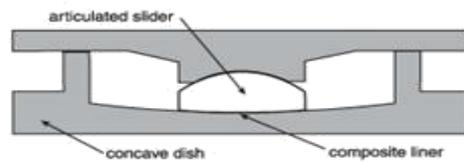
**Fig 11 Friction Pendulum Bearing**
