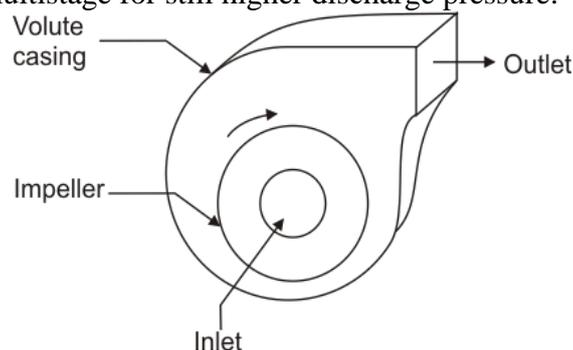
**Fig.2.1 A centrifugal fan or blower**
