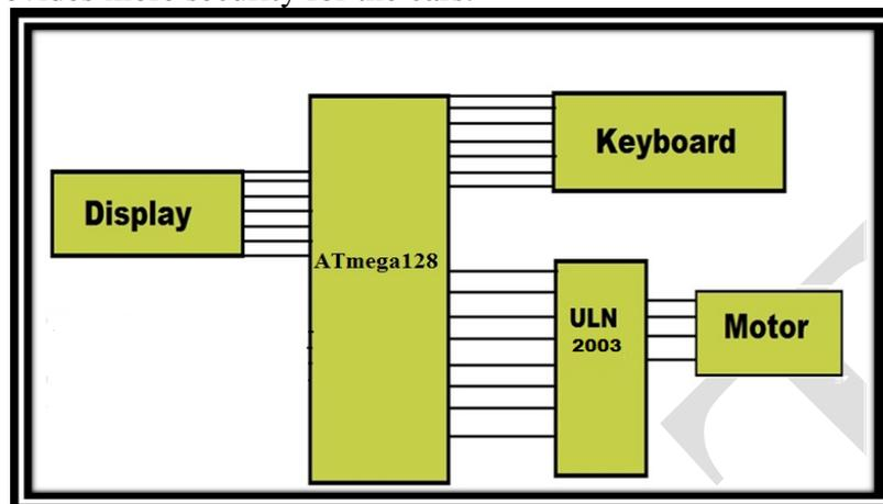
**Fig. Block Diagram of Car Parking System**
