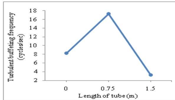
**Figure 5: Turbulent Buffeting Frequency vs length of tube**
