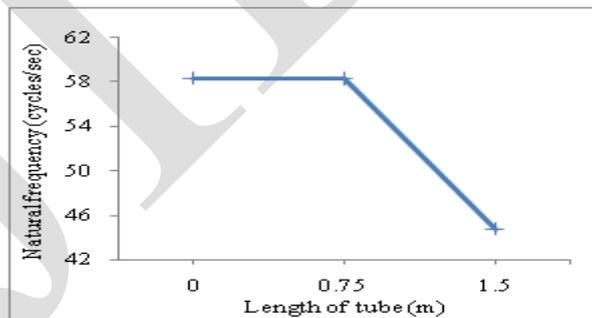
**Figure 3: Natural frequency vs length of tube**
