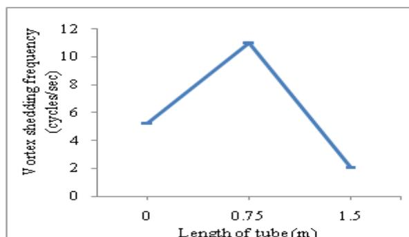
**Figure 4: Vortex shedding frequency vs length of tube**
