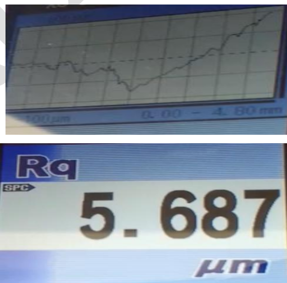
Fig.3.10. Surface roughness of a hole in dry condition
