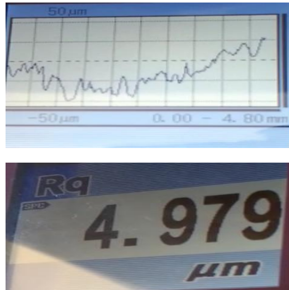
Fig 3.11. Surface roughness of a hole in HPCJ condition
