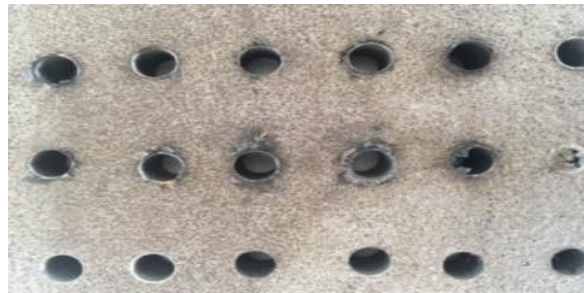
Dry condition (Roundness of the holes close to the end )
