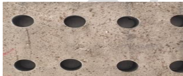
HPCJ condition (Roundness of the holes close to the end)
