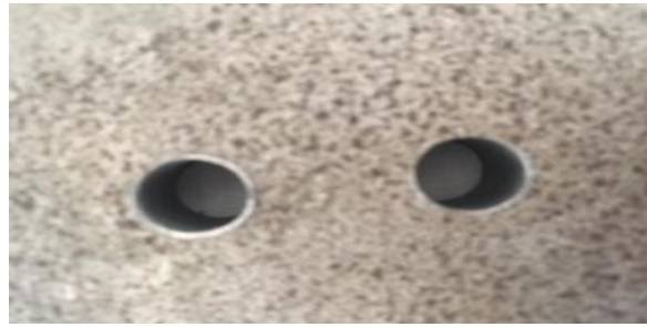
HPCJ Condition (Roundness of the holes close to the entrance)
