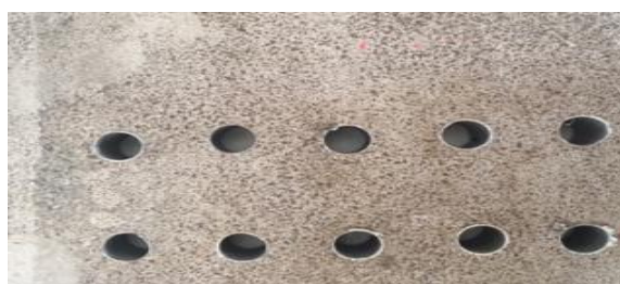
Dry Condition(Roundness of the holes close to the entrance) Fig:3.4
