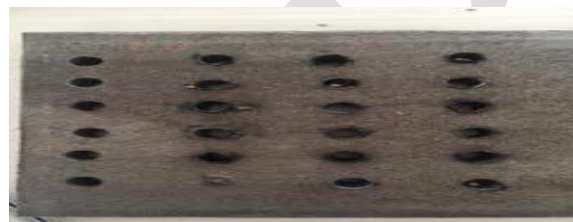
Holes drilled under Dry Condition
