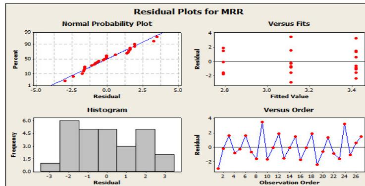
Fig.8 Residual plots for material removal rate versus feed, depth of cut
