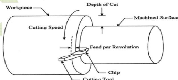
Fig. 1: Representation of figure during Turning Process
