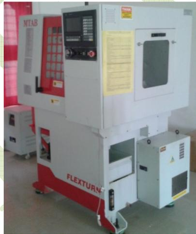
Fig 2 CNC vertical turning machine
