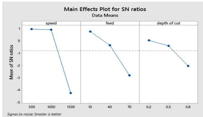
Fig .7 Most important effects plot for S/N ratio (surface roughness)
