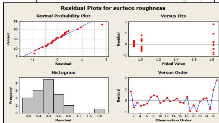
Fig .9Residualplots for surface roughness versus feed, depth of cut
