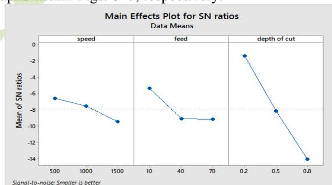
Fig .6 Most important effects plot for S/N ratio (material removal rate).
