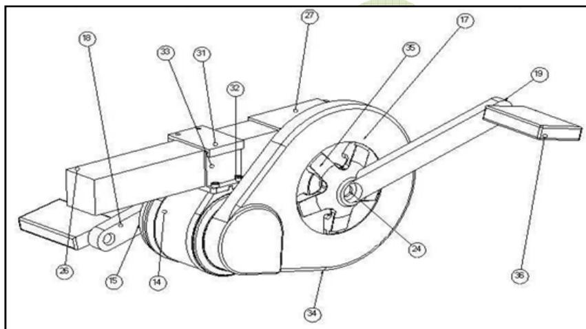
Figure 2: generator module. [11]
