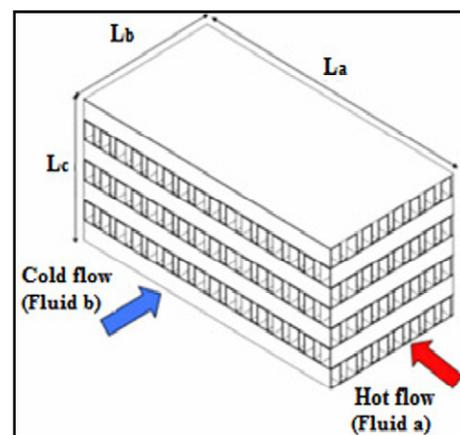
Fig. 2 Serrated Plate Fin Heat Exchanger (SPFHE) - For Air-Oil Cross Flow
