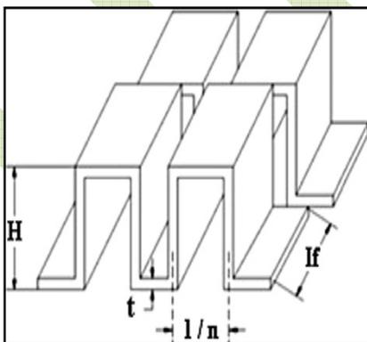
Fig.1 Serrated Fins
