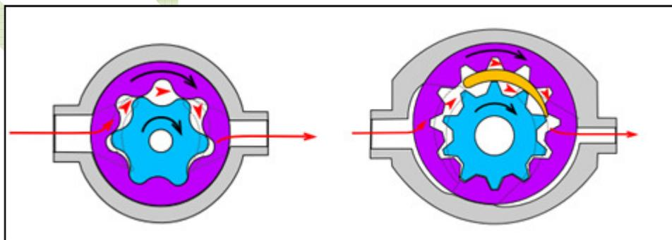
Fig. 1. Internal gear pumps with and without a crescent-shaped partition resp.
