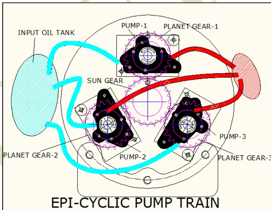
Fig. 3. CAD drawing of pump
