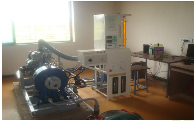
Fig 3 Four Cylinder Four stroke S.I. Engine Test Rig
