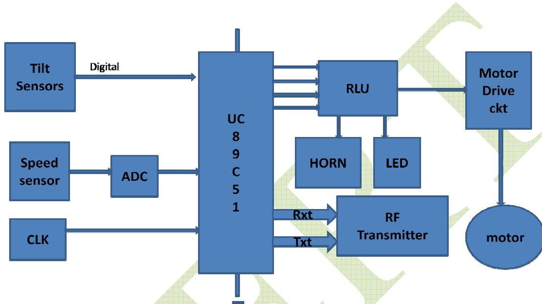
Fig1: Transmitter Unit
