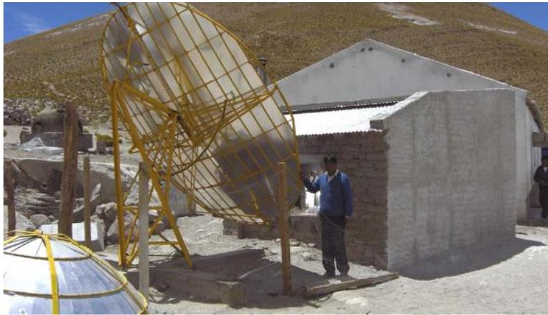
Figure 5: Solar community oven powered by Scheffler reflector
