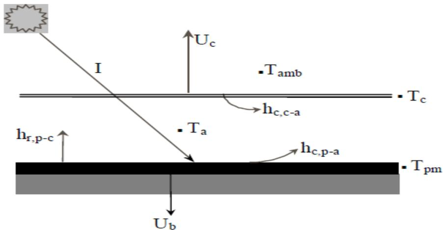
Figure 1: Flat-Plate Solar Collector Heat Transfer Parameters.
