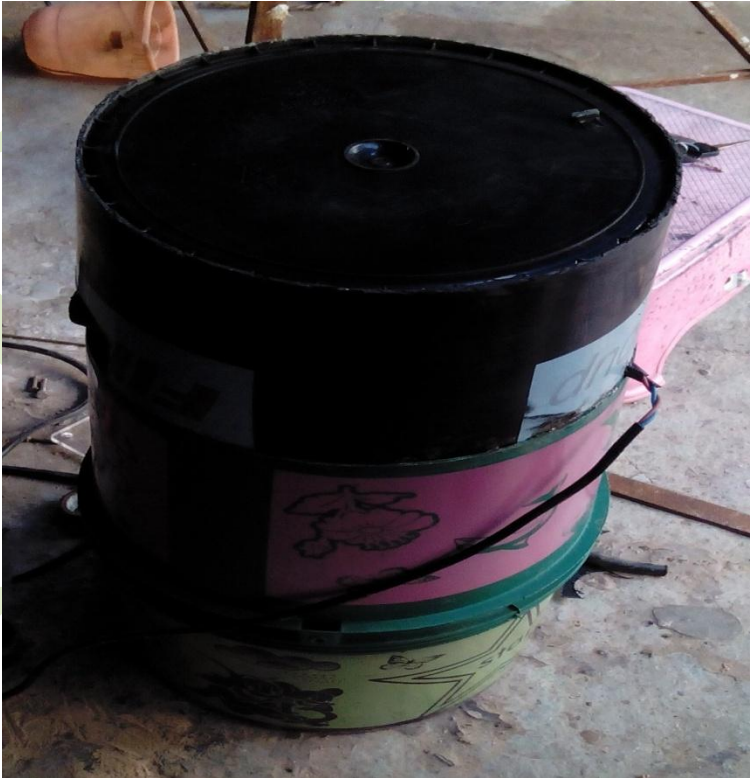
Figure 2: Bottom part of Dust Collector
