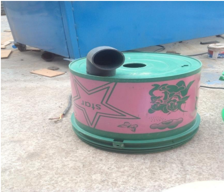
Figure 1: Top part of Dust Collector
