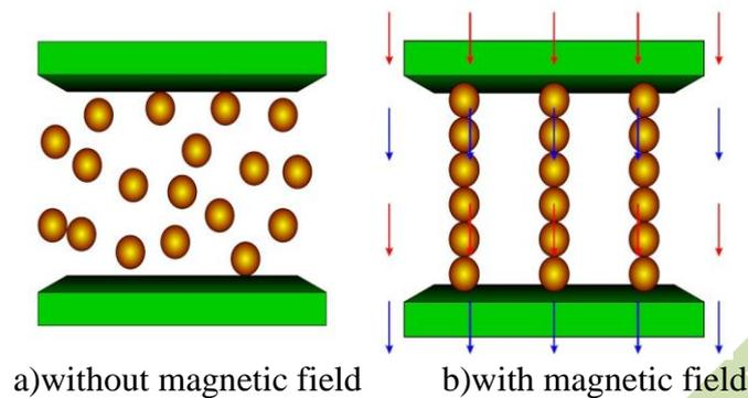
Fig.1. Working principle of MR fluid technology
