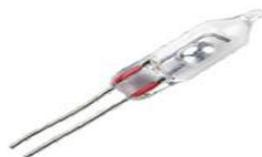
**Fig (3): Tilt Sensor[1-5]**
