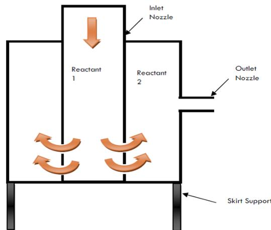
Fig. Block diagram of Reactant Column
