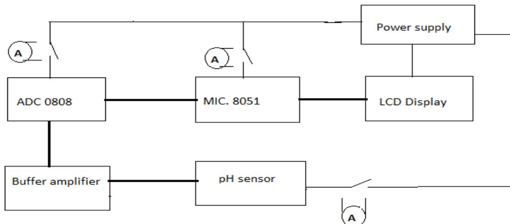
**Fig.1 Block diagram of microcontroller based pH measurement**
