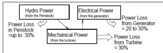
Figure shows that some power is lost at each stage during the conversion from a water jet to electricity
