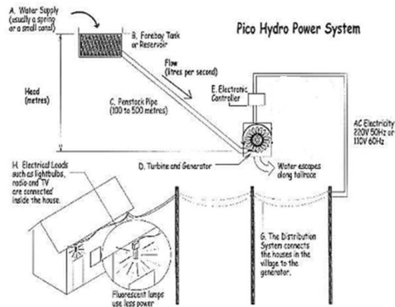
**Figure shows the layout of a picohydro system.**
