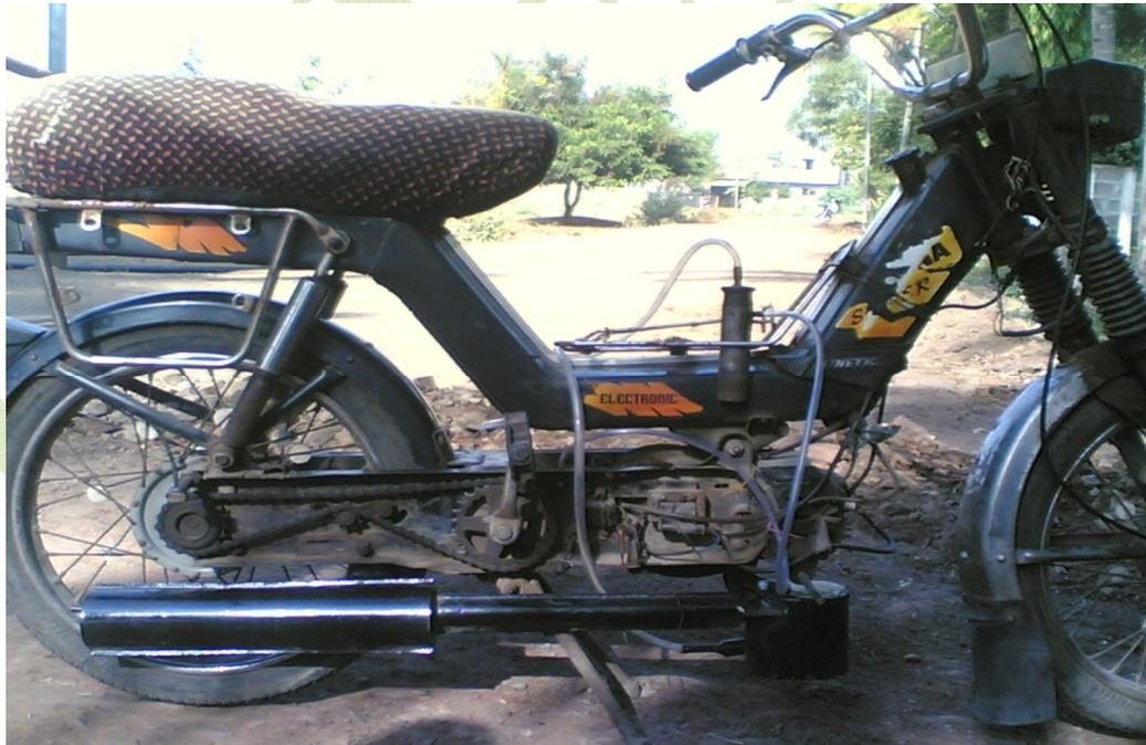
**Fig: Fabricated Turbocharger With Engine Arrangement**
