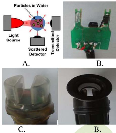
**Fig.2 Turbidity sensor. (A) Measurement principle. (B) Probe board. (C) Flat surface PTFE housing. (D) Inline Tee fitting**
