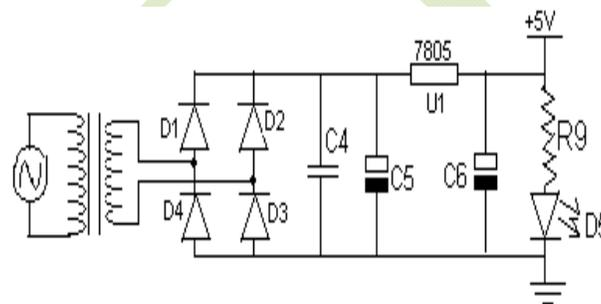
Fig. 5 Power Supply Circuit
