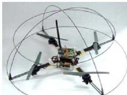
**Fig2. Quad rotor vehicle with frame protector.**
