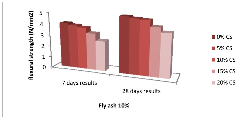
**Figure 3: Flexural strength of concrete with different replacement levels of cement with copper slag for 10% fly ash**
