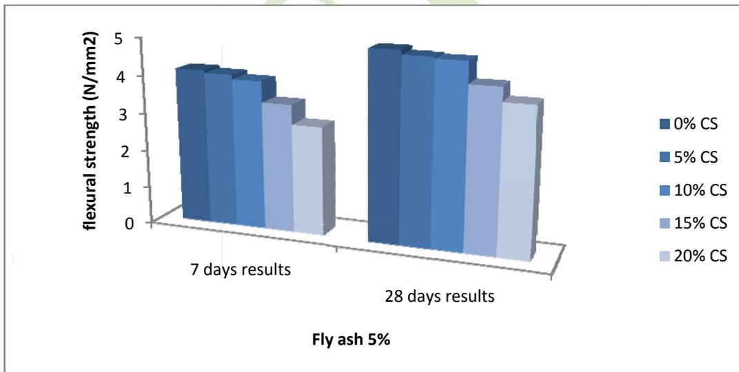
**Figure 2: Flexural strength of concrete with different replacement levels of cement with copper slag for 5% fly ash**
