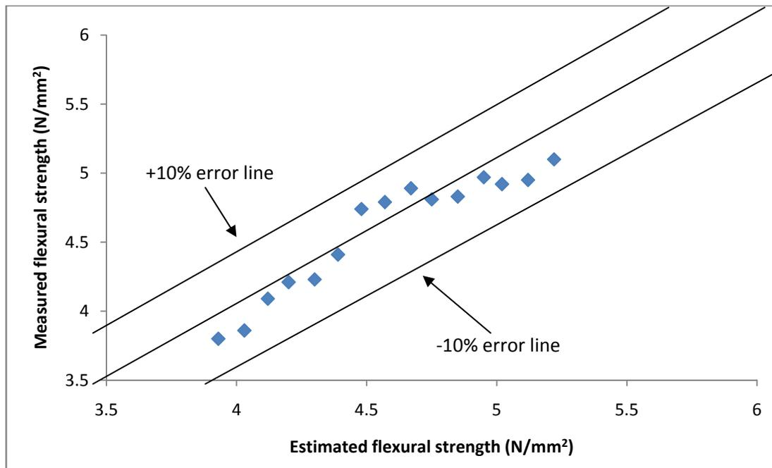
**Figure 4: Variation of estimated flexural strength and measured flexural strength for different mixes**
