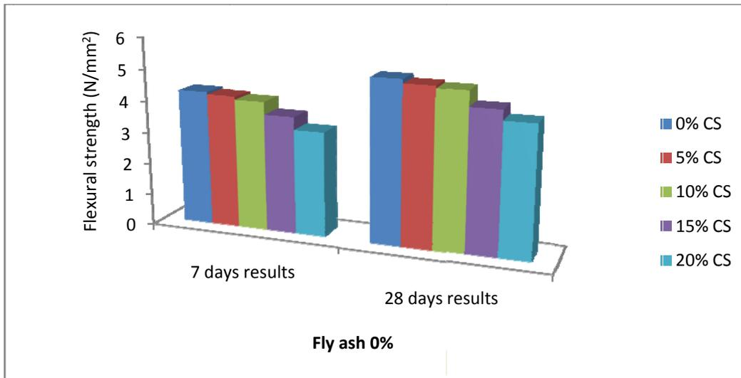
**Figure 1: Flexural strength of concrete with different replacement levels of cement with copper slag for 0% fly ash**
