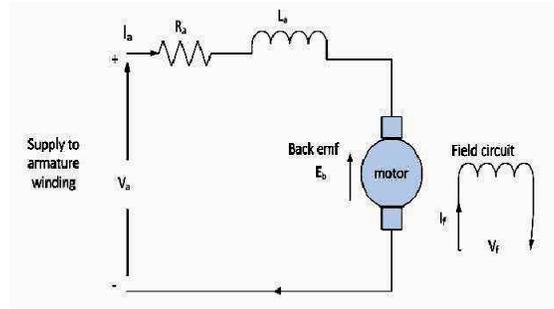
**Figure 1: Schematic Diagram of a separately excited DC Motor**
