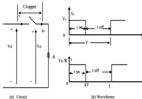
**Figure 3: Operation of chopper and its waveforms**
