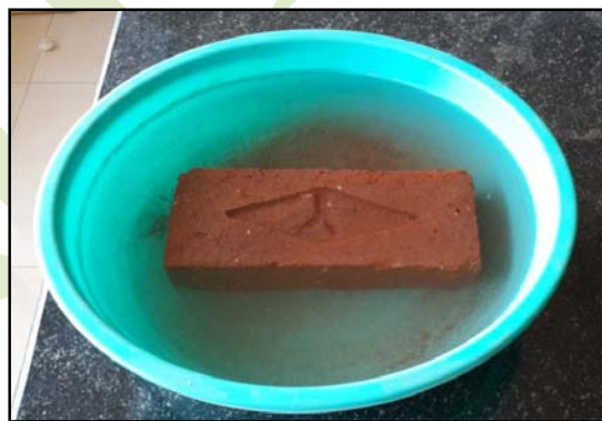
Figure 3: Water Absorption Test
