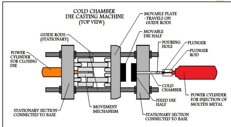
Fig.1. Pressure Die Casting Machine.
