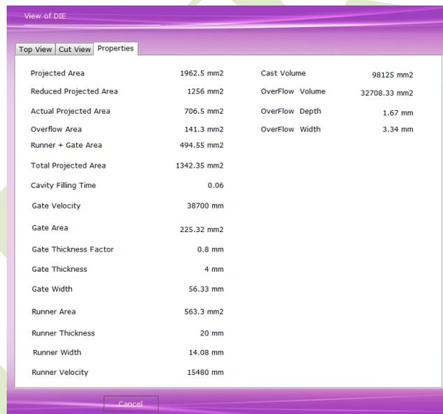
Fig. Output parameters of software.
