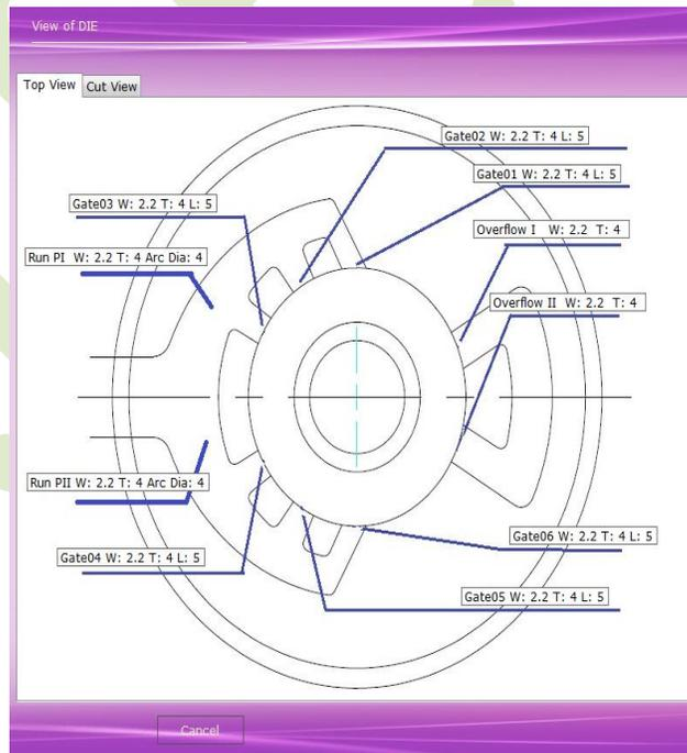
**Fig. Top View Output parameters of software.**
