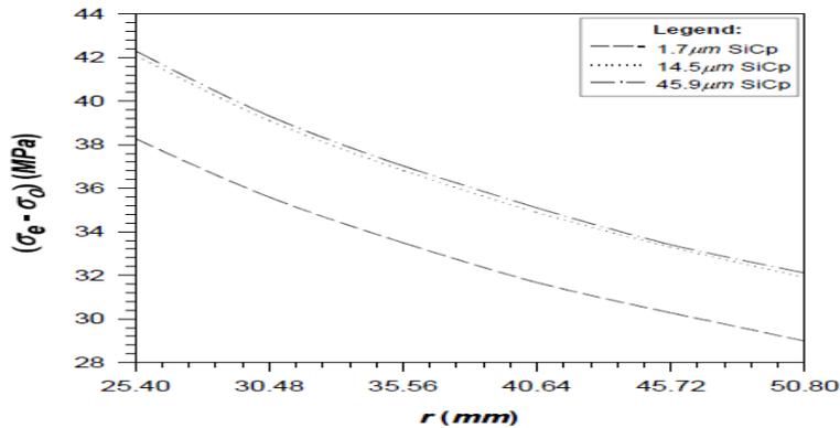
Fig No. 5 Variation of stress difference for varying particle size of SiC ( $V = 10 \text{ vol}\%$ ,  $T = 350 \text{ }^\circ\text{C}$ ).
