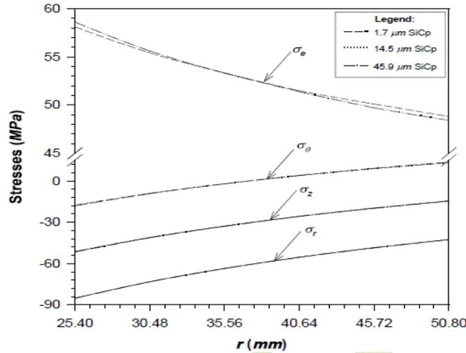
**Fig 3** Variation of creep stresses for varying particle size of SiC ( $V = 10 \text{ vol}\%$ ,  $T = 350 \text{ }^\circ\text{C}$ ).
