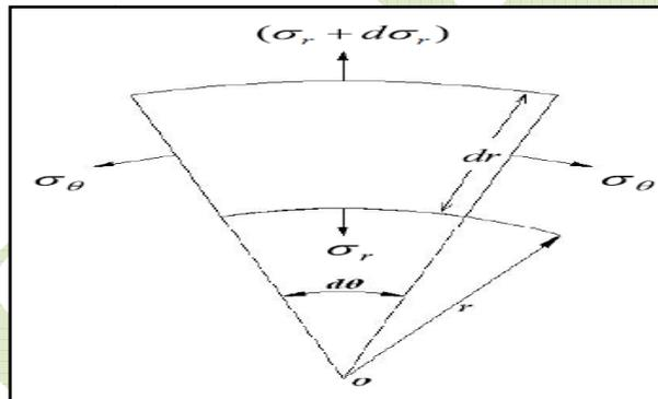
**Fig. No. 2 Free body diagram of an element of the composite cylinder**
