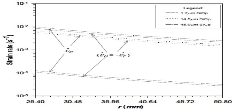
**Fig no. 4 Variation of strain rates for varying particle size of SiCp ( $V = 10\text{vol}\%$ ,  $T = 350\text{ }^\circ\text{C}$ ).**
