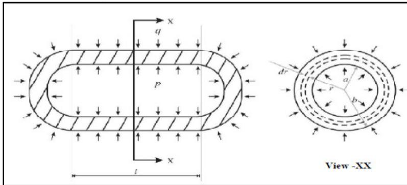
**Fig. No.1 Schematic of closed end, thick-walled composite cylinder subjected to internal and external pressures.**
