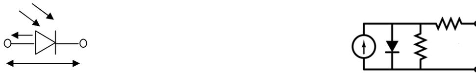
**Fig.4 Schematic symbol of solar photovoltaic cell Fig. 5 Equivalent Circuit of a photo cell**
