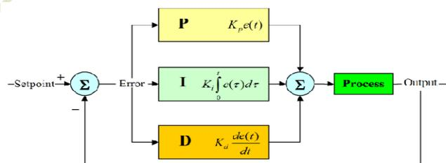
**Figure 3: PID controller block diagram**
