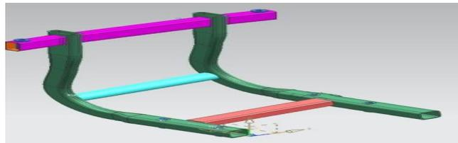
**Fig 1: Isometric view of the mounting bracket**
