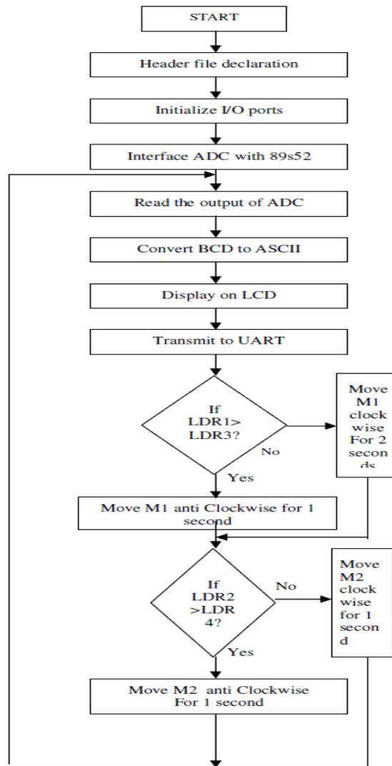
Figure 3: Software flowchart of automatic solar tracking system
