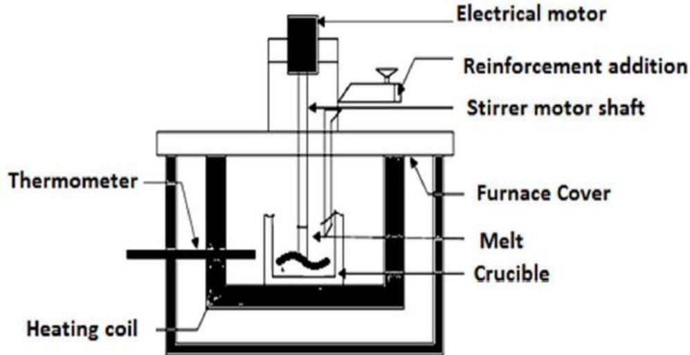
Fig 1 Schematic view of stir casting setup [7].
