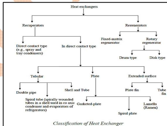
Figure 1 Classification of heat Exchanger
