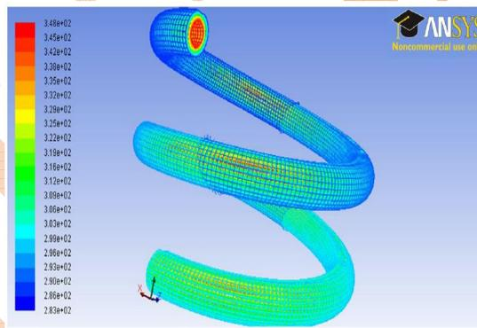
Fig 10 Contours of Static Temperature
