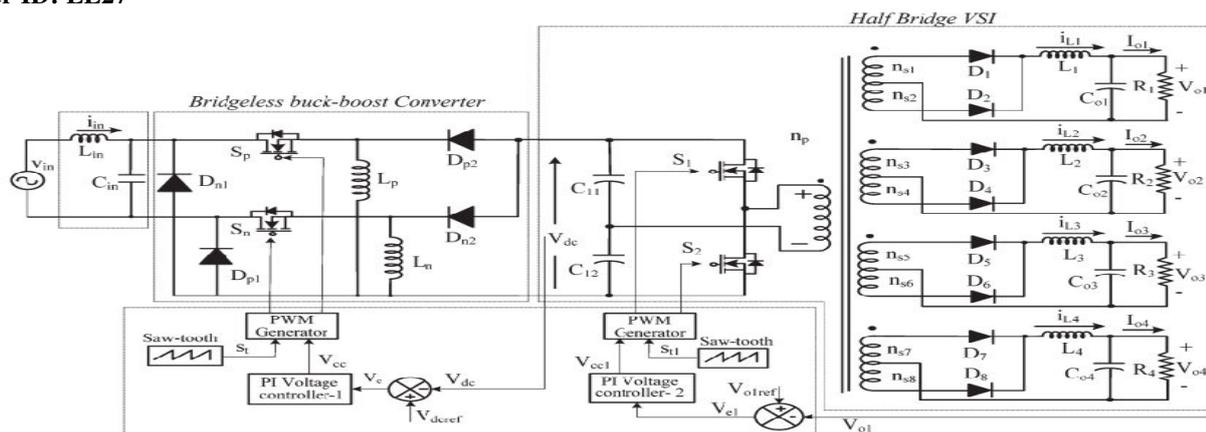
Fig 1-Circuit configuration of proposed multiple output switched mode power
