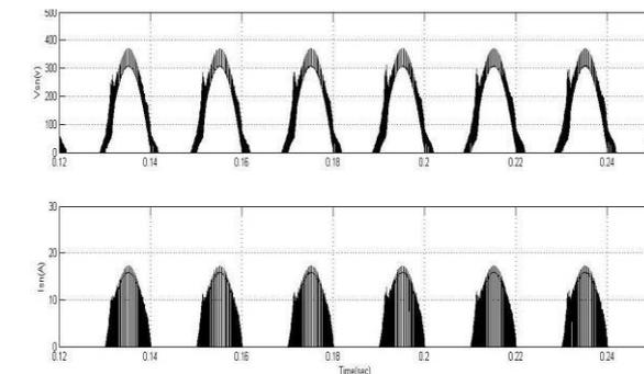
Fig 4 -Voltage across Switch Sp and Sn and Current through switches.
