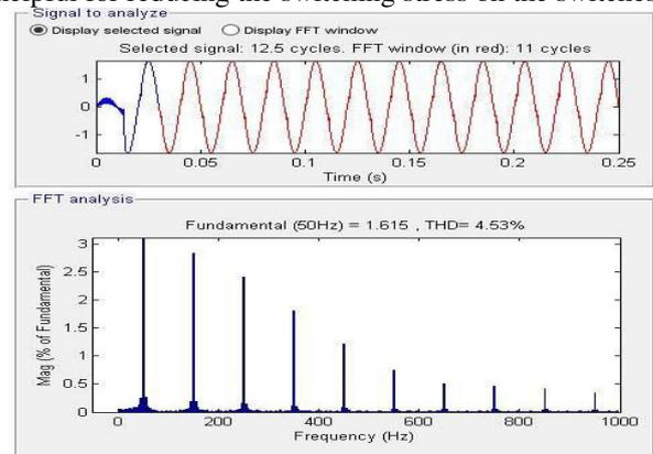
Fig 2- input ac current and harmonic spectrum
