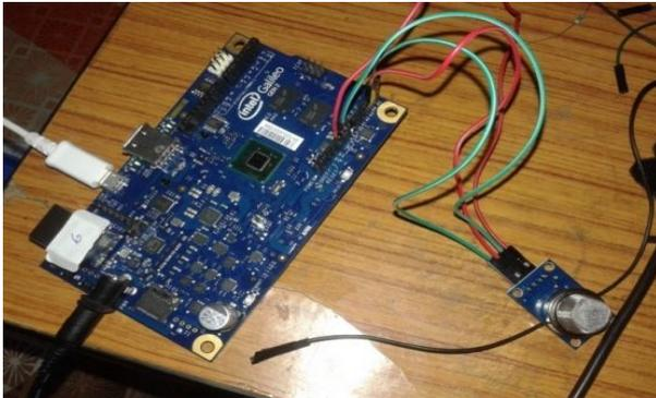
Fig-2 Interfacing diagram of gas sensor with Galileo gen 2 board
