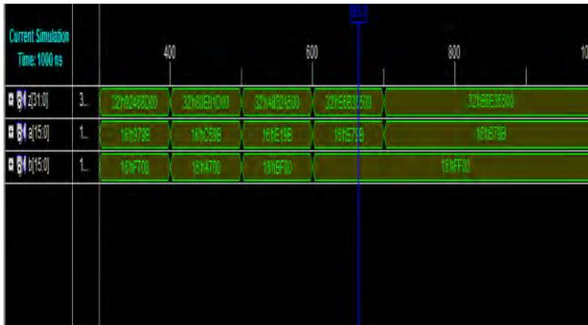
Figure 10: Simulation result of 16X16 bits Vedic multiplier(Nikhilam method) by ISE.
