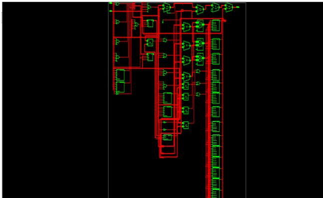
Figure 11: RTL view of 16X16 bits Vedic multiplier(nikhilam method)
