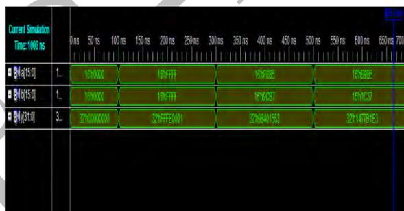
Figure 8: Simulation result of 16 × 16 bits Vedic multiplier by ISE
