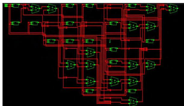
Figure 9: RTL view of 16 × 16 bits Vedic multiplier by ISE
