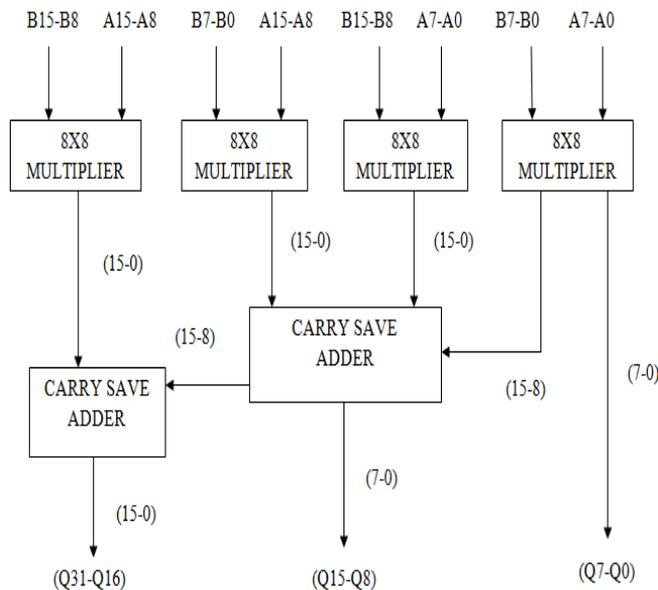
Figure 2: 16 × 16 Bits decomposed Vedic Multiplier
