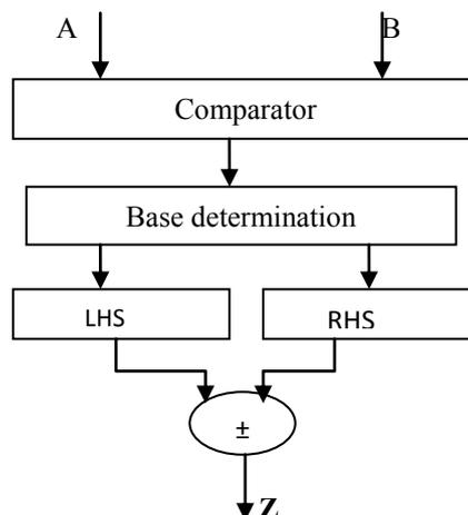
Figure 5: Block diagram of Nikhilam sutra
