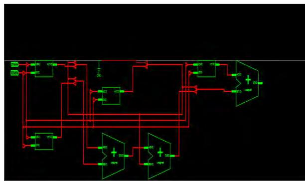
Figure 7: RTL view of 8 × 8 bits Vedic multiplier
