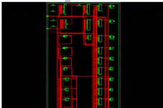
Figure 11: RTL view of 16X16 bits Vedic multiplier(nikhilam method using urdhva thirykbhyam)
