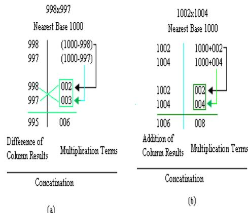
Figure 4: Procedure of multiplication using “Nikhilam Navatascharamam Dasatah” Sutra, (a) Numbers are taken below base, (b) Numbers are taken above base.
