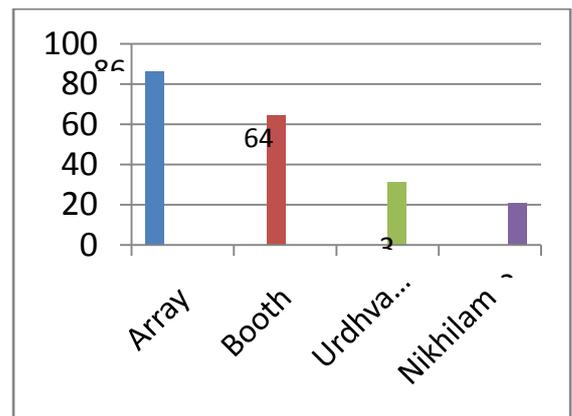
Figure.12: Time delay graph for various 16 bit multipliers
