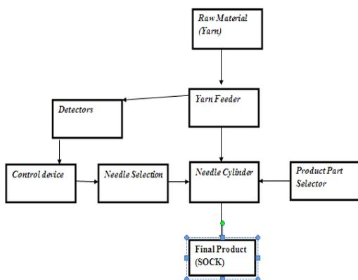
Fig.1. Block diagram of developed system
