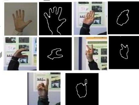
Fig. 5. Boundary Detection results of the proposed system for posture Five, B, C, V, and Point.
