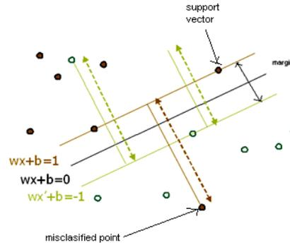
Fig. 2. Linear separating hyper-plane and Support vectors. The separation problem is to determine the hyper-plane such that  $x_i + b \geq 1$  for positive examples and  $w x_i + b \leq -1$  for negative examples.
