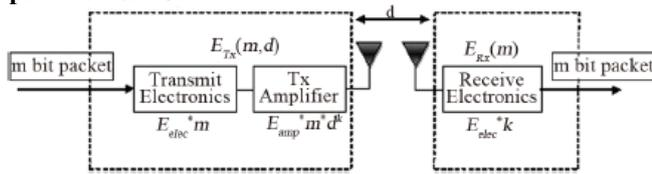
Fig. 5. Radio energy dissipation model [6]
