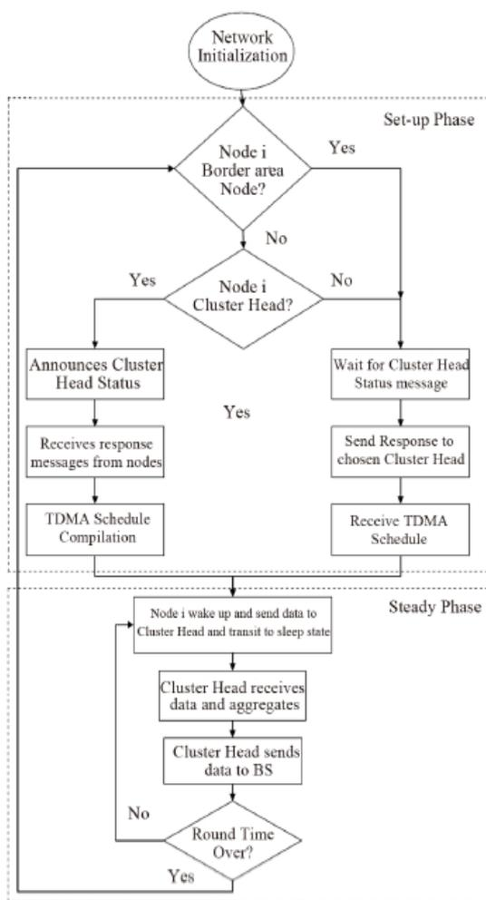
Fig: 4 Block diagram of clustering in SCHS [6]
