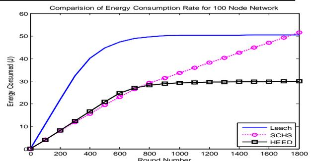
Fig. 7. Comparison of energy consumption rate of LEACH, SCHS and HEED.
