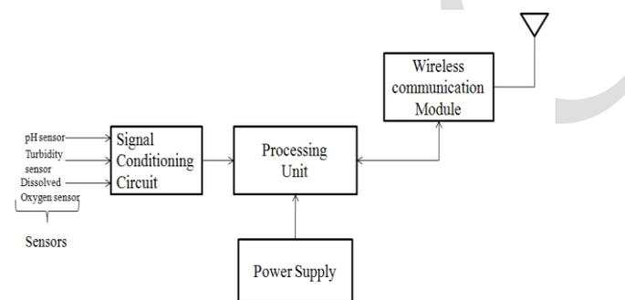
Fig2. Sensor Node Unit
