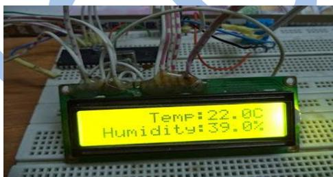
Figure-3 Display of result on LCD connected to microcontroller
