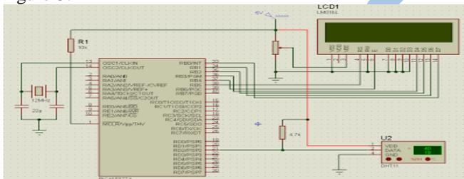
Figure-2 Schematic diagram of DHT11 interfacing with P16F877 PIC microcontroller
