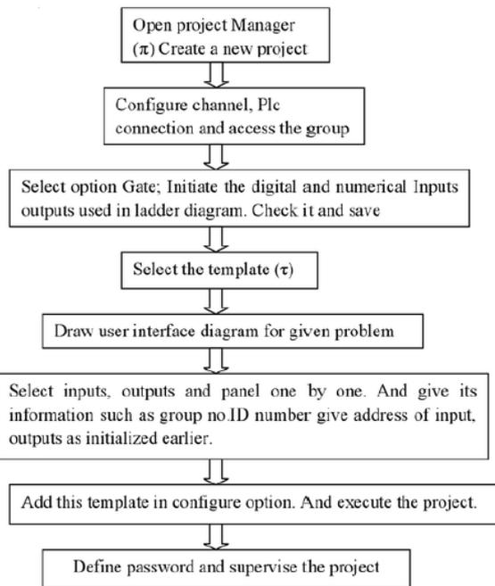
Figure-5 Flowchart of SCADA Template design using WinLog Lite software
