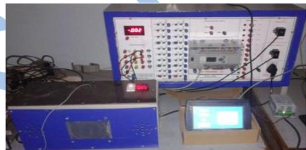
Figure-4 DHT11 interfacing with PLC Allen Bradley MicroLogix 1400 series
